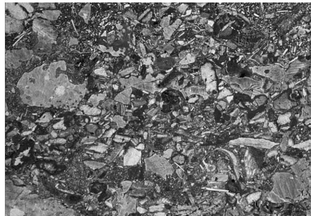
Fig. 3. Very poorly sorted bioclastic packstone composed exclusively of fragments from the calcitic shell layer of rudists. Note that the preservation of the shell fragments ranges from angular, unmicritized to rounded with a micrite rim; note also macroborings in some of the fragments. This packstone is the matrix of a rudist biostrome with an open to packed, parautochthonous rudist fabric. Upper Santonian, Gosau, Austria. Width of view 12 mm.
