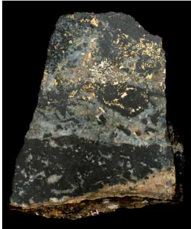
Fig. 5. Banded mineralization of chalcopyrite and pyrite in tourmaline (black) and quartz. Vecchia Bedovina-M. Mulàt mine. The maximum length of the sample is 8cm.
