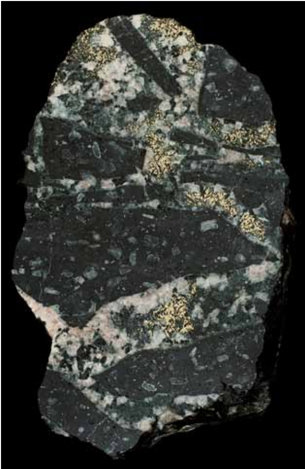
Fig. 4. Volcanic clasts, cemented by quartz veins with K-feldspar and chalcopyrite. Bedovina mine. The maximum length of the sample is 11cm.
