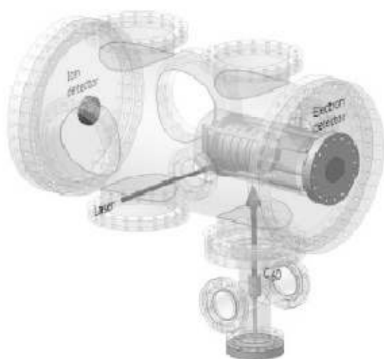
Fig. 1. Schematic picture of the VMI spectrometer setup
