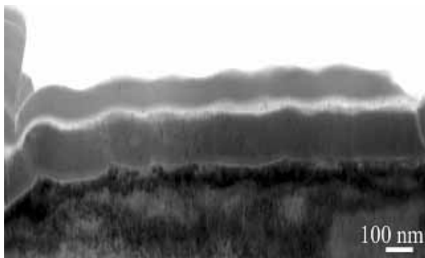
Fig. 3 TEM cross section of TiB_2 coating deposited on steel substrate.
