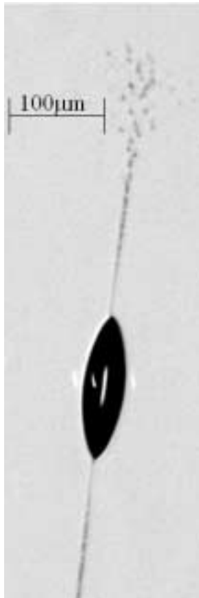
Fig. 1: Microphotograph of an liquid droplet in the moment of coulomb instability. The two Rayleigh – jets are clearly visible. The droplet is rotationally symmetric around its long axis.
