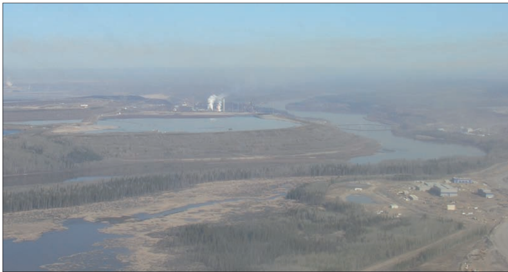
Fig. 1: Aerial view of the Athabasca Oil Sands area with visible air pollution emissions from the Suncor Oil Sands Plant (May 2005). Brown horizontal haze in the background is caused by emissions from the Syncrude Oil Sands Plant main stack. The Athabasca River crosses the landscape while the water body in front of the Suncor Oil Sands Plant is a tailings pond (Photo courtesy Andrzej Bytnerowicz).
