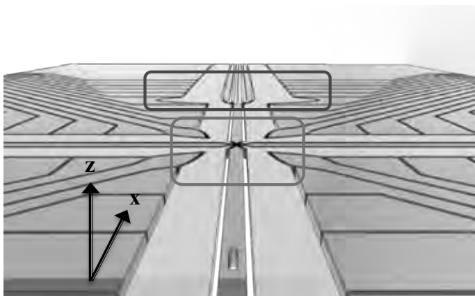
Fig 1) The structure of the multi-functional ion trap chip.
