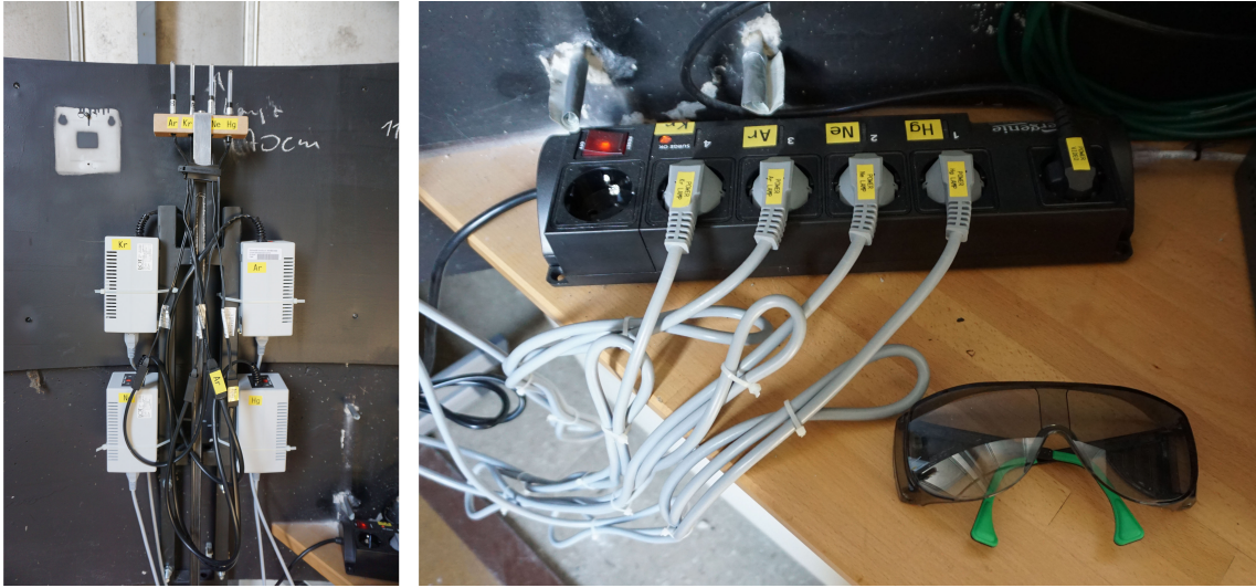
Figure 4: Penray lamp array. Left: Penray lamps at the movable holder; Right: Power supply for the lamps (individually remotely controllable). Note that some of the lamps have strong UV emission. Use the shown protection glasses!
